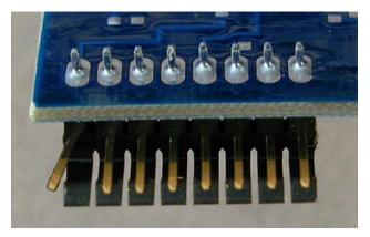
Figure 34 Bent Pin on Control Board
