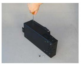
Figure 6 Side Screw Removal (part 1)
