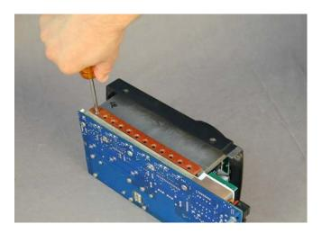
Figure 44 Installing FET Bar Screws
