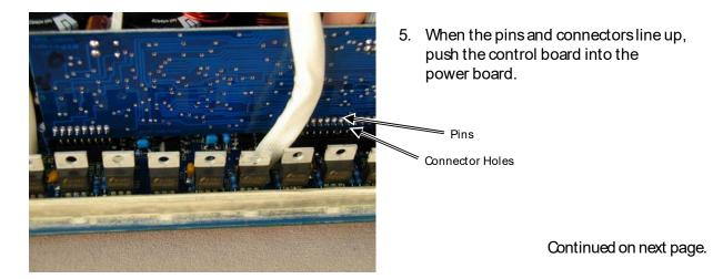
Figure 36 Pins and Connectors
