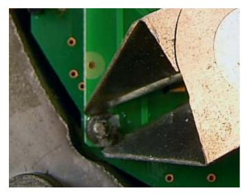
Figure 25 Gripping the Push-nut
