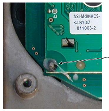
The button board is mounted to the heat sink on four metal pegs at the corners of the board. It is retained in place by push-nuts which slide over each peg, and which are covered in turn by silicone sealant.
