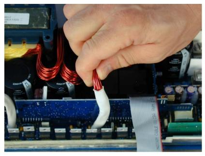
Figure 39 Placing Inductor Wires
