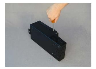
3. Replace and tighten down all the screws on the sides of the chassis.
