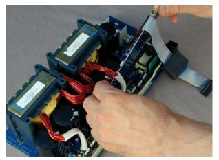
Figure 33 Sliding the Control Board Out
