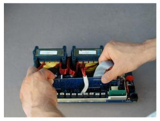
Figure 35 Inserting Control Board
