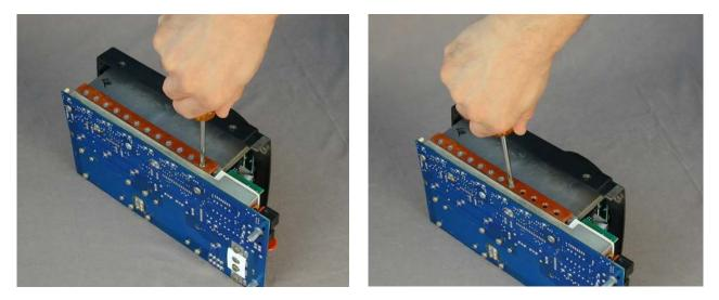
Figure 9 FET Bar Screw Removal
