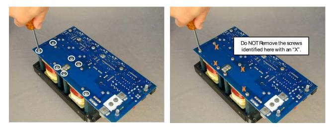
Figure 13 Bottom/Cradle Screw Removal
