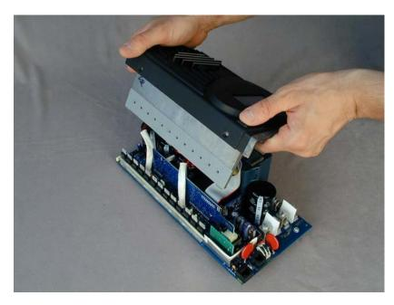
3. With all the screws removed, the heat sink can be separated from the power board. Set the unit upright and carefully pry and lift the heat sink off the power board.
