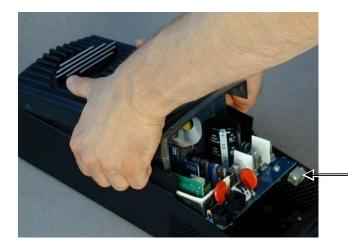
1. Side the reassembled unit into the chassis working around the Grounding lug.
