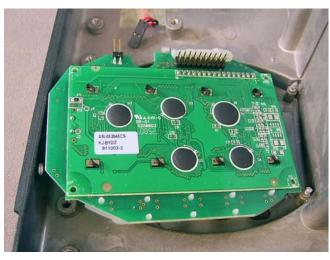
Figure 29 Inserting the New Button Board
