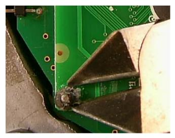
Figure 26 Deforming the Push-nut
