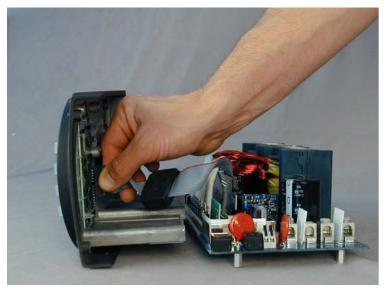
Figure 17 Cable Removal
