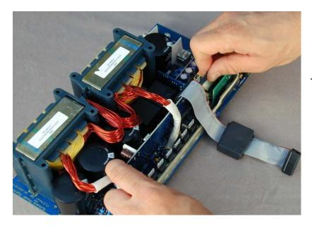
1. Push on both ends of the control board to confirm it is still properly seated on the power board.
