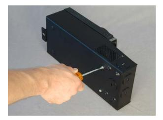
2. Replace and tighten down all the screws on the back of the chassis.
