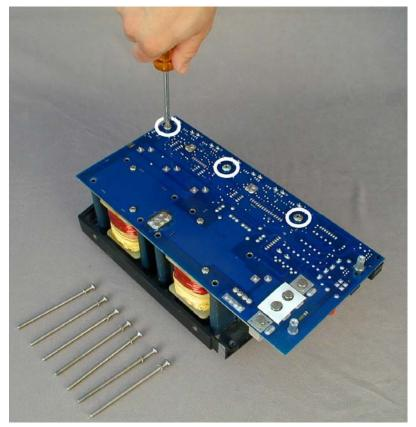
Figure 14 Removing Remaining Screws
