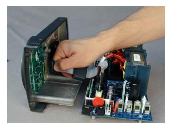
Figure 40 Reinstalling Ribbon Cable
