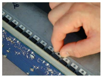
Figure 11 Freeing the FET from the Insulator
