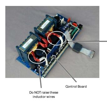
Figure 32 Lifting the Inductor Wires
