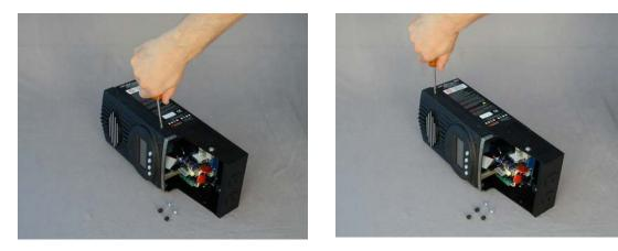
Figure 7 Side Screw Removal (part 2) The heat sink can now be removed from the chassis.
