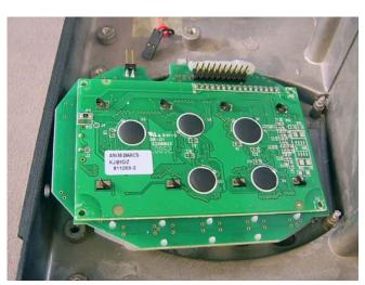
Figure 28 Removing the Button Board
