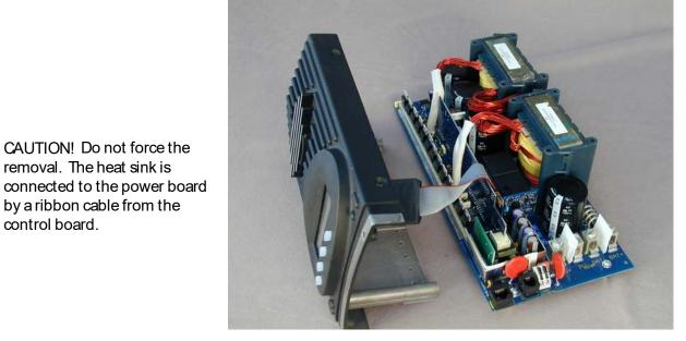
Figure 16 Heat Sink Connected to Power Board
