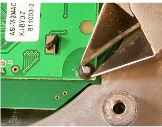
Figure 30 Inserting New Push-nut
