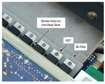
6. Using the replacement that came with the new board, replace the gray SI-Pad insulator on the heat sink.
