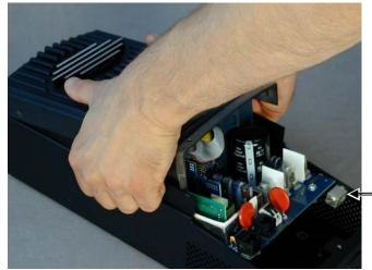
1. To remove the heat sink, grip it along each flank and raise its lower end.
