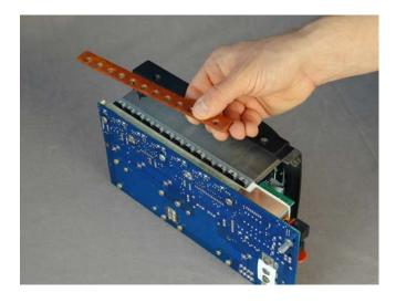
6. Set the unit on its side with the FETs in between the screw holes on the heat sink.
