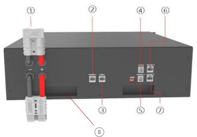
(1): Positive and negative connector \* 2 - for battery parallel connection and power output, model: Anderson 120A
